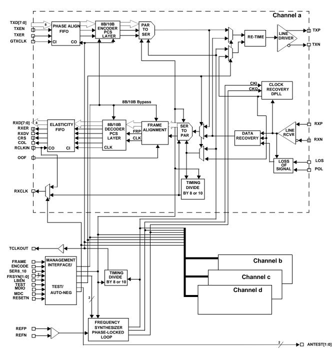
Figure 3. CYP32G0401DX Transceiver Block Diagram
