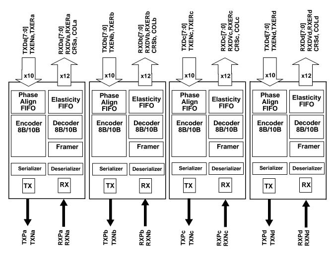
Figure 2. CYP32G0401DX Transceiver Logic Block Diagram
