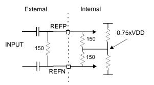
Figure 7. Reference Clock Termination
