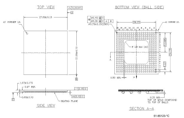
256-Lead L2 Ball Grid Array (27 x 27 x 1.57 mm) BL256
